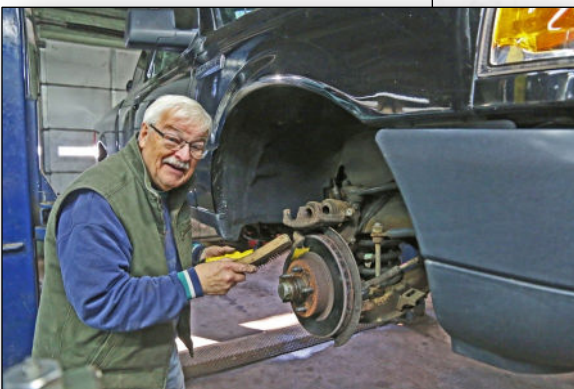
Don replacing the brakes on his Ranger Pickup Truck at a club Saturday morning workshop.
